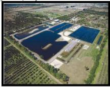
Though monitoring continues, the project has estimated reductions of Total Suspended Solids at 203,251 kg/yr, Total Phosphorus at 5,169.6 kg/yr (35% of the basin's loading), and Total Nitrogen at 17,124.5 kg/yr (20% of the basin's loading).
